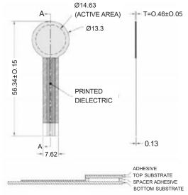
SECTION A-A LAYER STACK-UP
